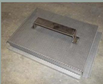
7. Pump inlet screen must be removed and cleaned thoroughly.
