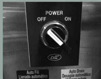
1. With Auto Drain: Push the auto drain button then wait 10 seconds and turn off the power switch.
