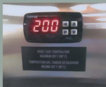
8. Make sure rinse tank temperature reaches 200 F (96 C).
