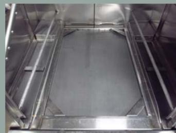
3. Position scrap trays in proper place and put floor grates in washer.
