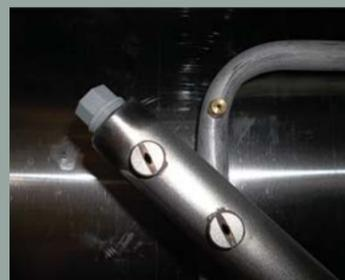
6. Wash and rinse nozzles must be inspected for blockage and cleaned.
